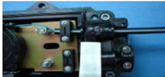
(3) Fix the optical fiber to splice case and coil the rest of the optical fiber inside splice case base and Fix the optical fiber to down body
