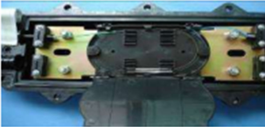
(3) Fix the optical fiber to splice case and coil the rest of the optical fiber inside splice case base and Fix the optical fiber to down body
