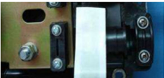
(5) Seal the unused ports by plugs.
